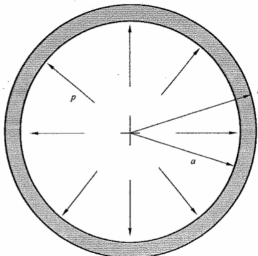
$$S_{\text{ta}} = p(b^2 + a^2)/(b^2 - a^2) \quad S_{\text{ra}} = -P$$
